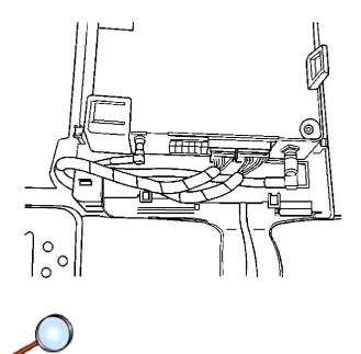
3. Install the module to the upper bracket ensuring the retaining tab is fully seated.
